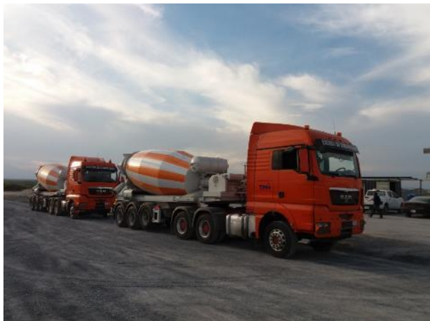
2 Hormigoneras Semi-remolque LIEBHERR HTM 1204 -12 m3
